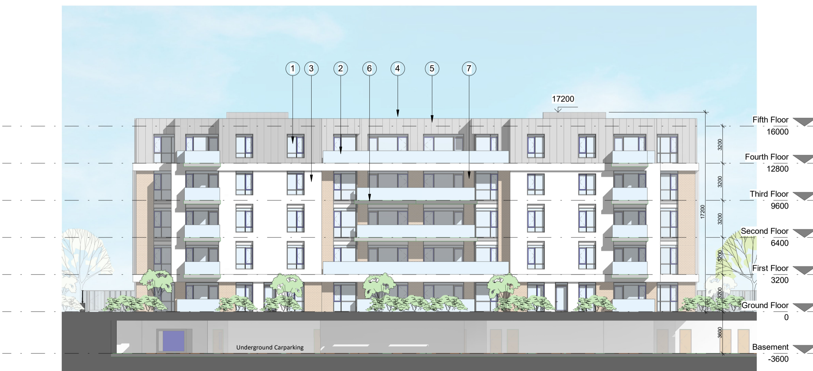
Block 2 South Elevation
